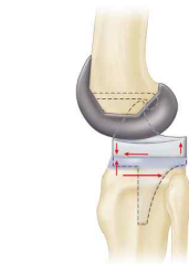
FIGURE 7-15 One argument against posterior cruciate ligament substitution is that added prosthetic constraint may ultimately transfer more stress to prosthesis-bone interface.
